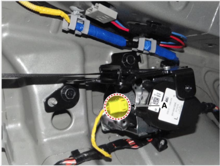
3. Remove the rear seat belt retractor (A) after loosening the mounting bolts.
